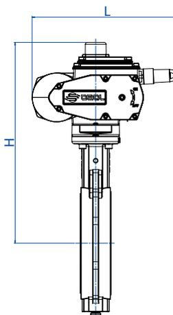
**CON ATTUATORE ELETTRICO ON-OFF - LENTE IN CF8M**
