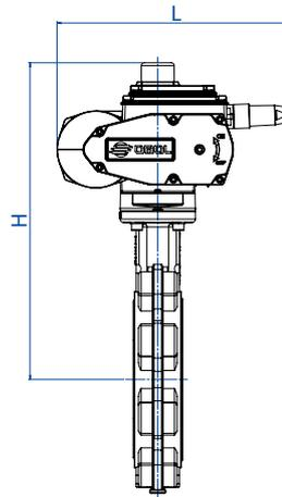
**CON ATTUATORE ELETTRICO ON-OFF - LENTE IN CF8M**
